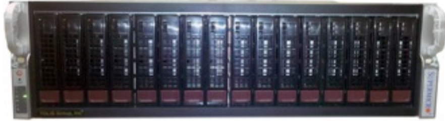
Figure 6.3 — Front view for the bruAPP 3U chassis. Power button and LEDs are on the lower left side of the chassis, just under the rack handle.
