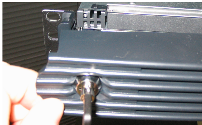
Fig. 6.1 — Removal of the 1U chassis faceplate/bezel if applicable.
