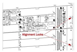
If you encounter resistance, adjust the upper module so that the alignment mechanism pin moves into the mating hole in the lower module.
