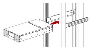
**3.** Tighten the **recessed screws** only one turn to hold it until it can be aligned with the other modules.
